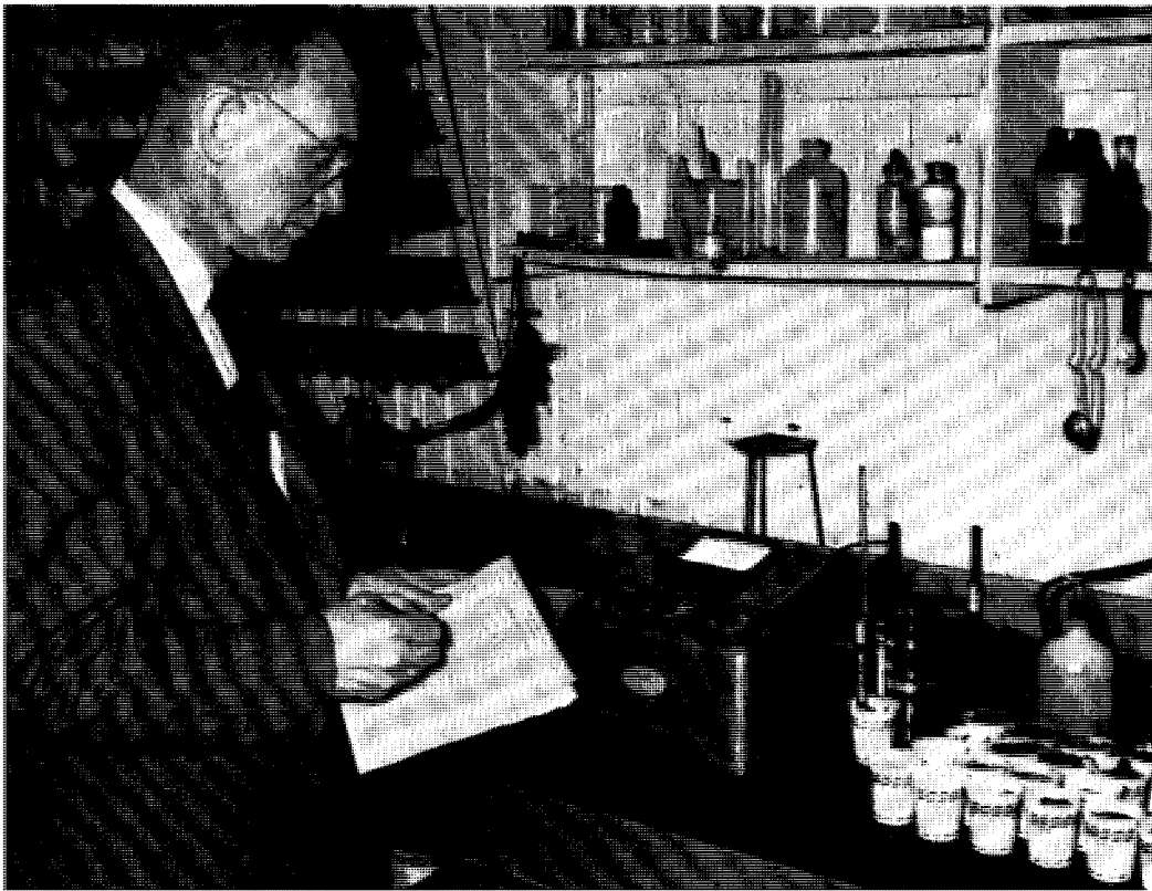
pH meter is probably instrument most widely used in soil laboratory. This model, the Beckman H-2, tests 25 ml. soil with enough water to make a thin mud. Electrode is placed in sample and reading made after 15 to 20 seconds
