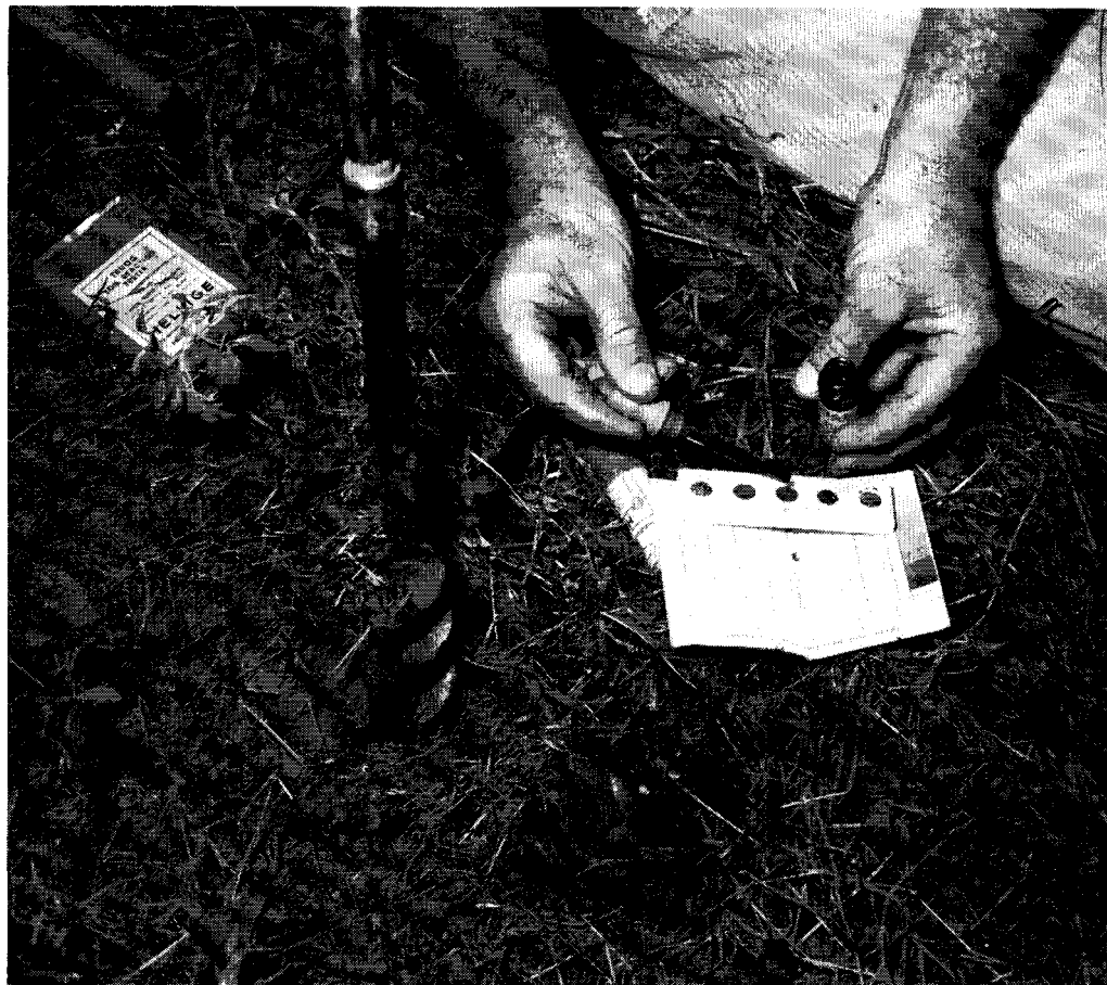
While well-developed laboratory equipment makes pH determination precise, simple color tests are used in the field for general indications
